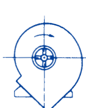
右回轉斜左下向 O Clockwise Bottom Angular Down
