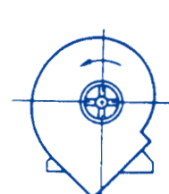
左回轉斜右下向 P Counter-Clockwise Bottom Angular Down
